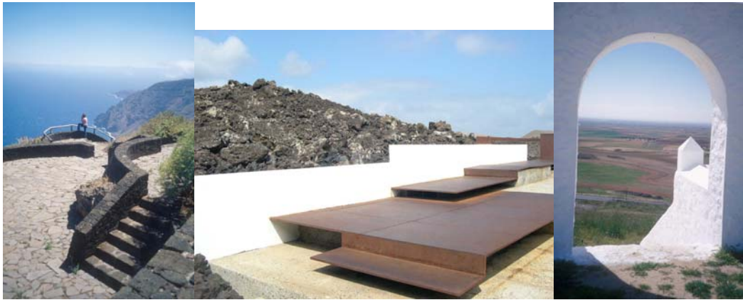
Fig. 56, 57 and 58. Scenic viewpoint facilities design. (Left) Stone parapets, stairs, lanes and standing areas displayed on a slope at different levels. (Centre) Rust steel, white parapet and badlands lava rocks make up the scenic viewpoint facilities. (Right) White clay and sand walls, stairs and arch frame the view. (Photos by I. Español)
