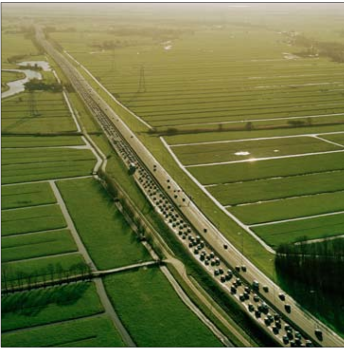
Figure 8.6 The A2 corridor at Vinkeveen, Netherlands respects the local historic landscape type both horizontally and vertically utilising the grain of the historic dyke drainage pattern. © Aerophoto-Schiphol
